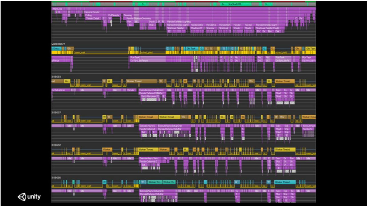
Previous execution where we had the main thread do a lot of the command logic (in this picture each row is a core.) and there were a ton of holes in rendering execution
