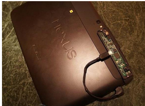
Capri depth camera attached to a mobile devices
