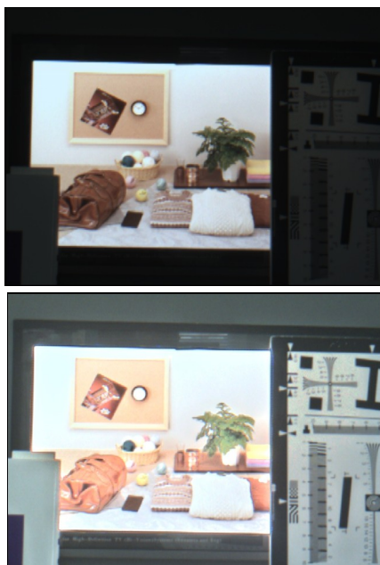
Figure 2: (top) A input image (14 bit) and (bottom) the result of WDR compression (8bit).
